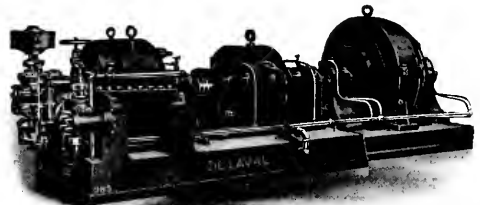
De Laval 300 K. W. Multi-stage Geared Turbine Driving D. C. Generator; built for U. S. S. "Arizona"
